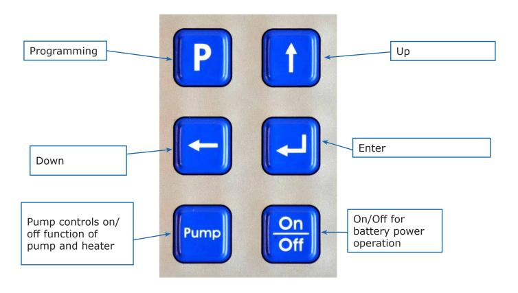
The keyboard is user-friendly and allows for function display changes even with work gloves or welding gloves. Through the audible "click" of the operation keys, choices are confirmed. The WS Oxy I can be programmed for a variety of functions, including audible and visual settings.
