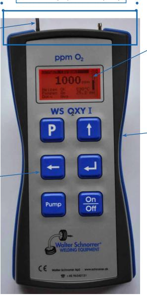
Multi colored graphic LCD display for all menus. Different colors indicate specific stages of the unit's operations.
