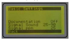
In the menu "Basic Settings" the values for the "Signal Sound" and "Signal ppm", which are visual and acoustic alerts, can be changed. "Documentation" can also be turned on or off.
